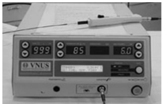
Fig. 2. The RF generator is shown here. The displays from left to right are RF generation time, temperature, impedance, and power in watts.
